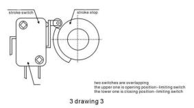
KST-20/50/100/200 The layout drawing of KST-20/50/100/200 stroke stop and stroke switch (drawing 4)
