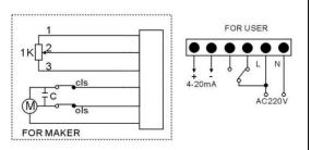
The opening or closing is realized by switching \*lose\* the circuit outputting a group of full open or close active signals.
