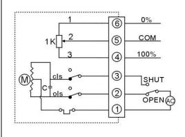
The opening or closing is realized by switching \*lose\* the circuit outputting a group of full open or close active signals.
