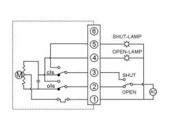
The opening or closing is realized by switching \*lose\* the circuit outputting a group of full open or close active signals.
