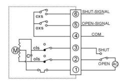
The opening or closing is realized by switching \*lose\* the circuit outputting a group of full open or close active signals.
