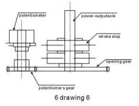
valve achieve  $10\Omega$ , tighten opening gear, fixing screw.(if the seven-line connector of regulate type are connected, please measure the resistance between RV and RS jacks.)
