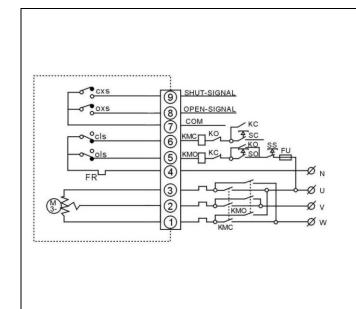
The opening or closing operation is realized by switching "open" or "close" the circuit "outputting" a group of full open or close passive signals
