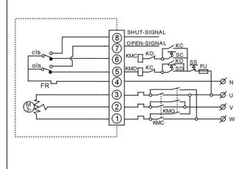
The opening or closing operation is realized by switching "open" or "close" the circuit "outputting" a group of full open or close passive signals
