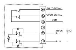
According to the single conductivity of diode, the opening or closing operation can be realized bye means of the exchanging of the positive polarity and the negative polarity and the negative polarity of DC power supply and output a group of full open or close passive signals.
